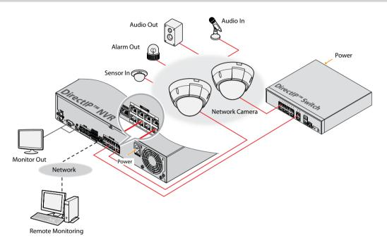
DirectIP<sup>™</sup> NVR makes it easy to use cameras without extra network configurations. Each camera can be controlled via the DirectIP<sup>™</sup> NVR setup menu, without any PC. For detailed camera settings, please see the camera setting pages of DirectIP<sup>™</sup> NVR manual.
