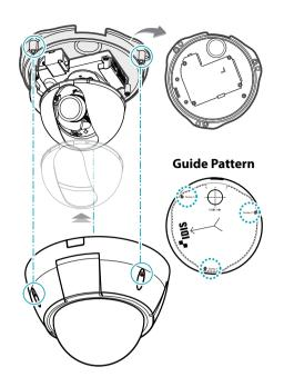
1 Use the screws provided with the camera to secure the bottom cover on a wall or a ceiling.
