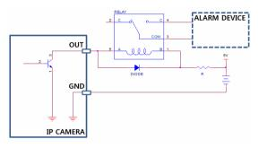
In: Connect an alarm-in device to this port. (Mechanism: Choose between an NC (Normally Closed) type or an NO (Normally Open) type) → Connect a mechanical or electrical switch to the alarm in port and the GND (ground) connector. Alarm in range is 0V to 5V. In order to detect alarm input from an electrical switch, the signal must be higher than 4.3V from an NC switch or less than 0.3V from an NO switch and must last for longer than 0.5 seconds.
