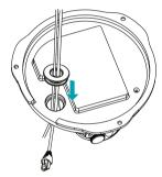
When using both network cable and wires of the power adapter, waterproofing sealing is required by using silicone etc. after blocking the cable access hole. Ask your retailer for details. 3 Use the screws, anchors provided with the camera to secure the bottom cover on a wall or a ceiling.
